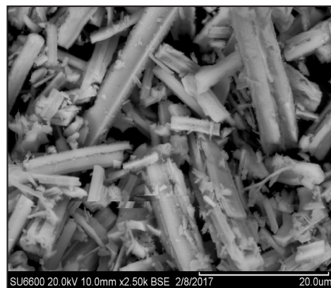
ZYP-55 is whisker shaped agglomerates of sub-micron particles.
