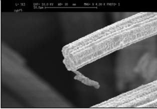
ZYBF-5 fibers are generally loose in nature with minimal fiber to fiber binding shown in the micrograph on the left. The micrograph on the right shows characteristically solid fibers with the grain size approaching a micron.
