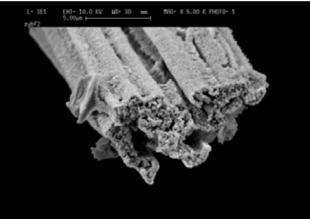
ZYBF-2 fibers are shorter than ZYFB-1 as shown in the micrograph on the left. It also shows significant fiber to fiber binding. The internal porosity and the sub-micron grains can clearly be seen at 5000x magnification in the micrograph on the right.
