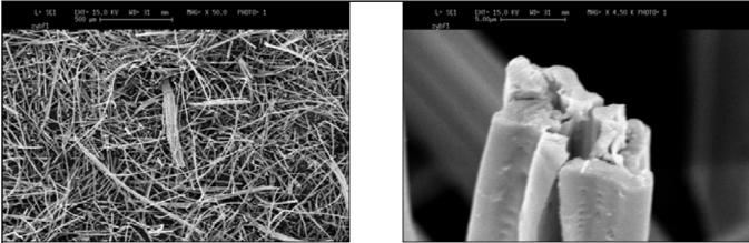
ZYBF-1 is the most reactive and has the highest shrinkage of our fibers. The fibers are generally long and loose as seen in the micrograph on the left. The micrograph on the right shows a fractured fiber with nano-sized crystalized grains that are not visable at that magnification.
